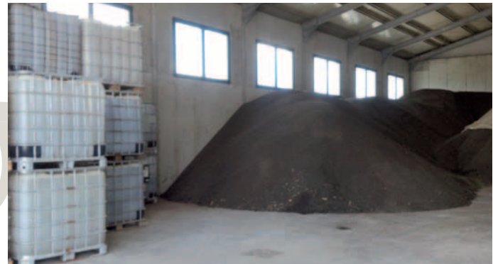
Figure 1 – Ammonium sulphate in 1,000 l bins and dried digestate.
