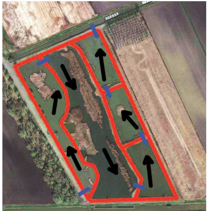
Figure 2 – The basins and channel after construction of the phytoremediation system.
