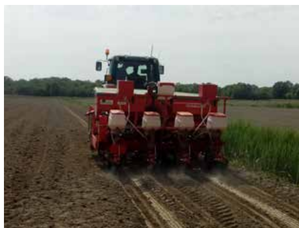
Figure 20 - Maize sowing with herbicide band application along crop rows
