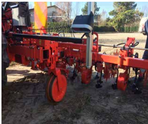
Figure 18 - Imaging camera that identifies crop rows and enables equipment position to be adjusted
