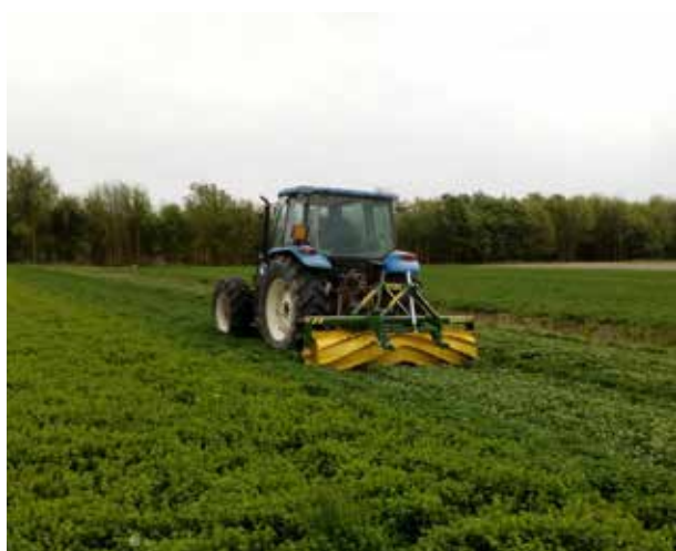
Figure 1 - Cover crop termination with Roller crimper
