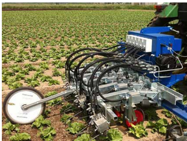
Figure 10 - Robovator developed for mechanical weed management, here in lettuce (photo by Frank Poulsen http://www.visionweeding.com/robovator/ )
