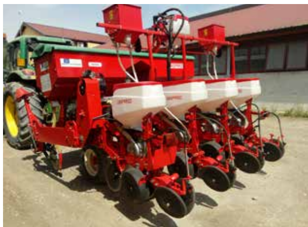
Figure 16 - Sowing machine equipped with nozzles for herbicide band application
