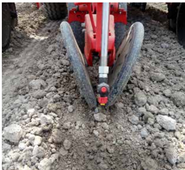
Figure 21 - Nozzle for herbicide band application positioned on the sowing machine
