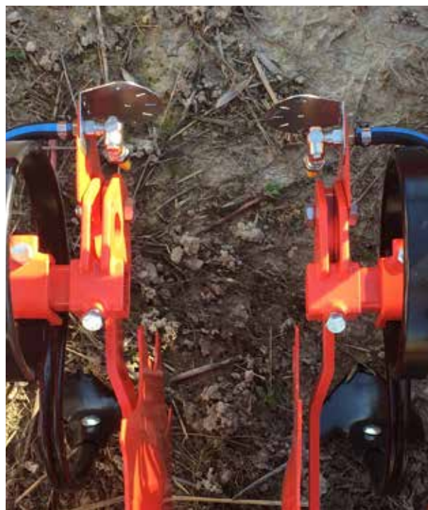
Figure 19 - Nozzles for herbicide band application along crop rows positioned on the cultivator structure
