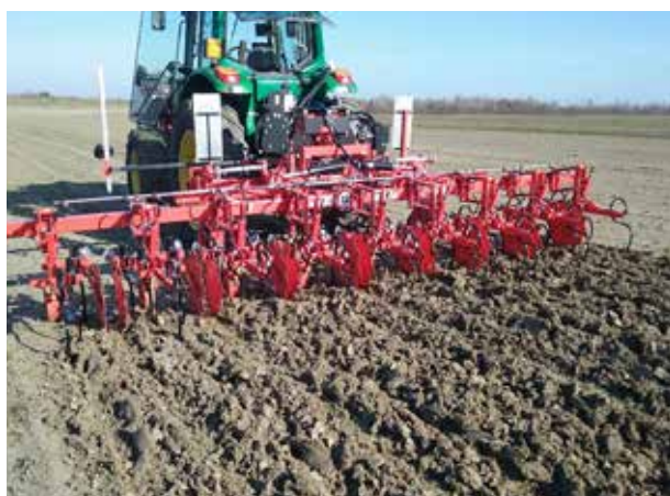
Figure 17 - The Maschio-Gaspardo prototype, which combines inter-row soil cultivation and herbicide band application along crop rows
