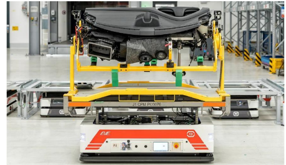
Figure 2: An example of mobile robot moving a dashboard in a factory shop floor[2]
