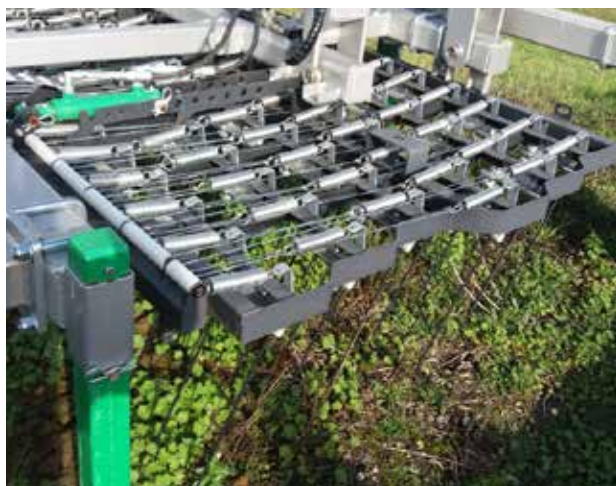
Figure 4 - Details of the precision tine harrow (Agronomic).
