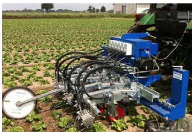
Figure 18 - Robovator developed for automated weed management, here in lettuce (Picture by Frank Poulsen, http://www.visionweeding.com/robovator/ ).
