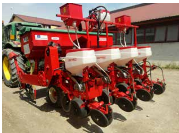
Figure 21 - Sowing machine equipped with nozzles for herbicide band application.
