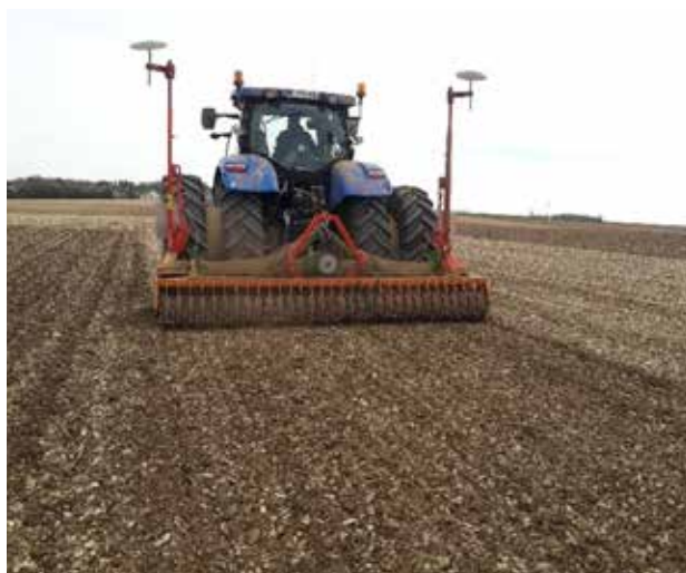
Figure 1 - Rotary harrow in Saint Michel's trial (24/04/2020) performed at 12 cm depth. Soil texture was very fine.
