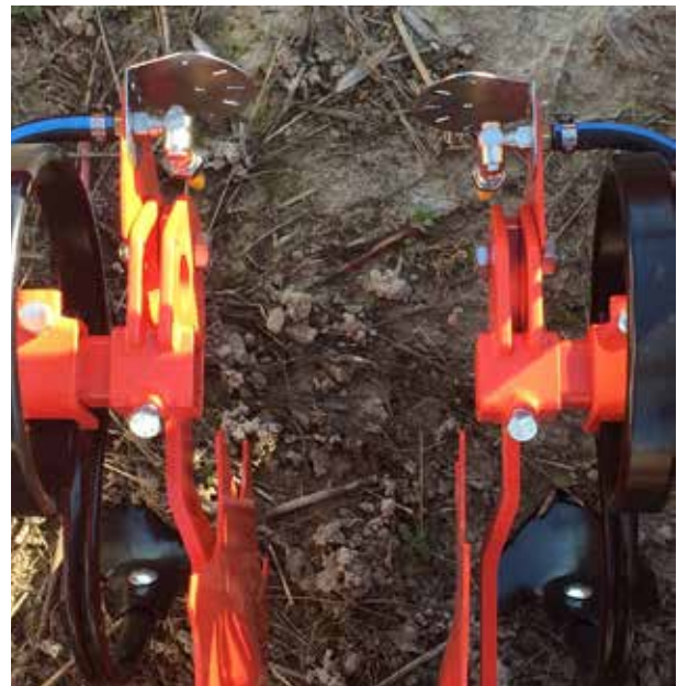
Figure 24 - Nozzles for herbicide band application along crop rows positioned on the cultivator structure.
