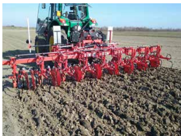
Figure 22 - The Maschio-Gaspardo prototype, which combines inter-row soil cultivation and herbicide band application along crop rows.
