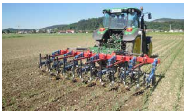
Figure 16 - First mechanical weeding in maize at the end of May 2020.
