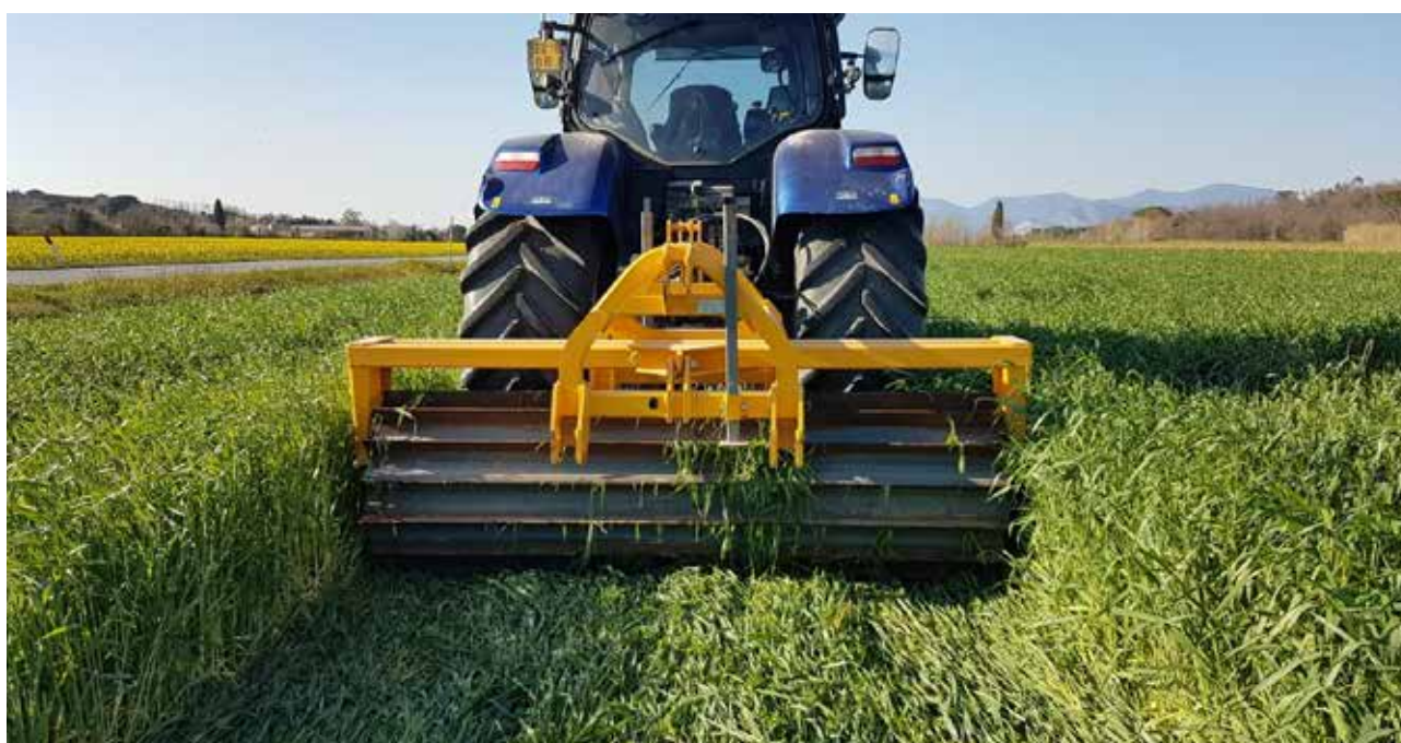
Figure 5 - Termination of rye by the cut-roller in 2018 at the full vegetation stage (first pass on 28 March).
