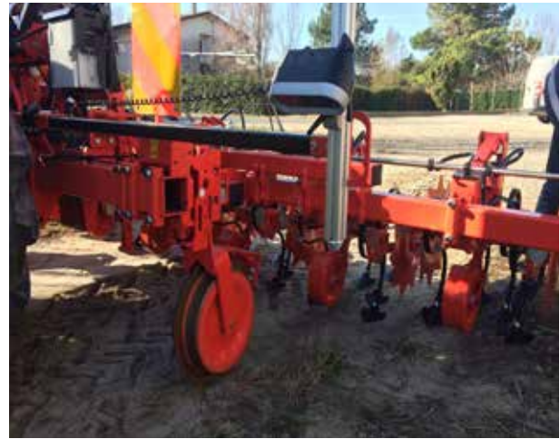
Figure 23 - Imaging camera that identifies crop rows and enables equipment position to be adjusted.
