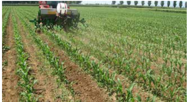
Figures 16 and 17 - Tine harrow (left) and inter-row cultivator (right) were used for mechanical weed control.
